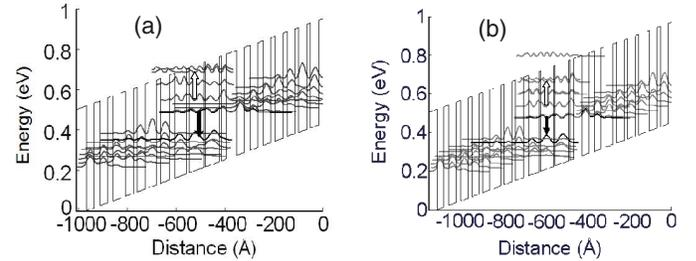
Fig. 1 Conduction band diagram of a portion of the active regions and injectors and the moduli squared of the relevant wave functions of a  $\sim 9.6 \mu\text{m}$  (a) and  $\sim 10.3 \mu\text{m}$  (b) QC lasers with a 4 quantum well active region. An electric field of 45 and 39 kV/cm is applied in (a) and (b), respectively. The solid arrows indicate the laser transitions. The open arrows represent pathways of resonant absorption
