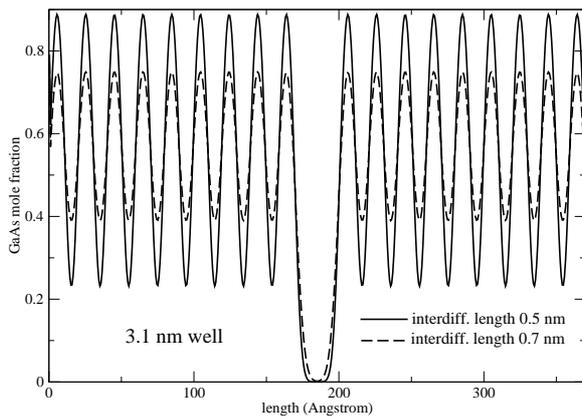
Fig. 2. The composition profiles of an initially rectangularly modulated all-binary GaAs-AlAs structure after interdiffusion.
