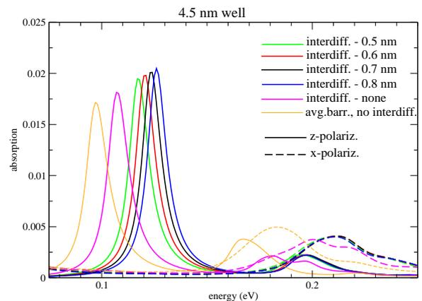
Fig. 1. The absorption profile evolution for the *p*-doped GaAs/AlGaAs superlattice-barrier quantum well structure described in [3] with variable degree of interdiffusion.
