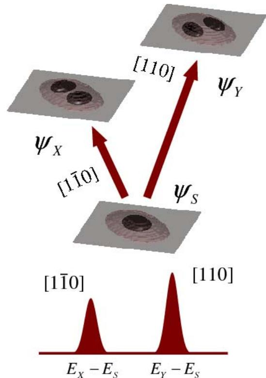
Figure 1. Schematic view of intersubband transitions from the ground electronic state  $\Psi_S$  to the first two excited states  $\Psi_X$  and  $\Psi_Y$  in an elongated self-assembled InAs/GaAs quantum dot. These transitions are respectively polarized along the long and short axes of the structure.
