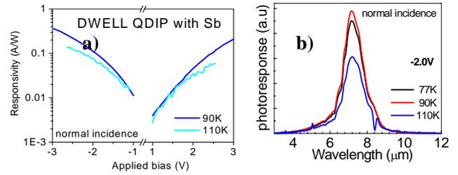
Fig.3. a) Peak Responsivity of DWELL QDIP with Sb at 90K(blue) and 110K(cyan) and b) Spectral photoresponse for DWELL QDIP with antimony at 77K(black), 90K(red) and 110K(blue) at normal incidence
