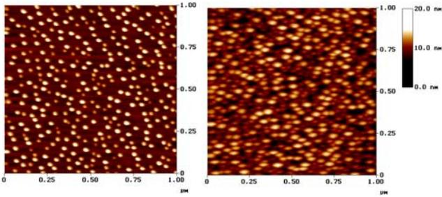
Fig.1. Atomic force microscopy images for conventional InAs /GaAs QDs (QD density  $\sim 4 \times 10^{10} \text{cm}^{-2}$ ) and InAs/GaAs QDs with Sb (QD density  $\sim 7 \times 10^{10} \text{cm}^{-2}$ )
