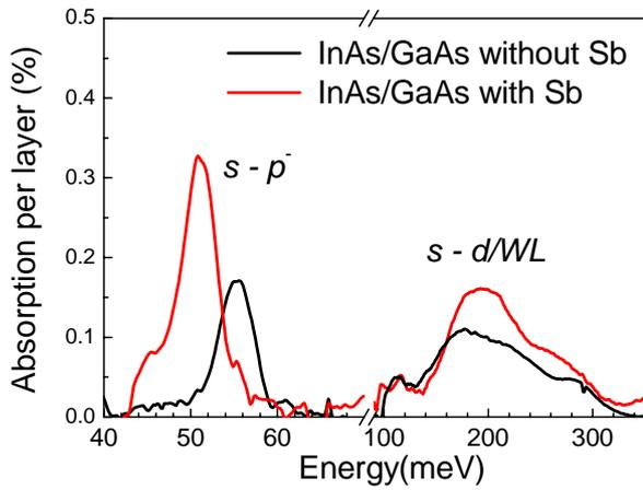
Fig.2. Absorption spectra for conventional InAs /GaAs QDs and InAs/GaAs QDs with Sb for samples with  $\sim 1$  electron per dot
