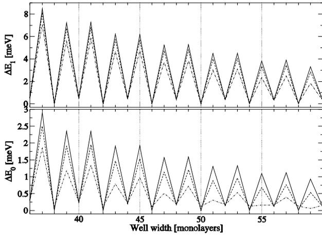
Fig.1: Valley splitting magnitude versus well width for the ground (bottom panel) and for the first excited (top panel) subbands of the QW system discussed in the text. Valley splitting for biased QW with field strength of 0.5 and 1.5 meV/Å are represented by dashed and dot-dashed lines, respectively. Solid lines refer to the zero electric field case.
