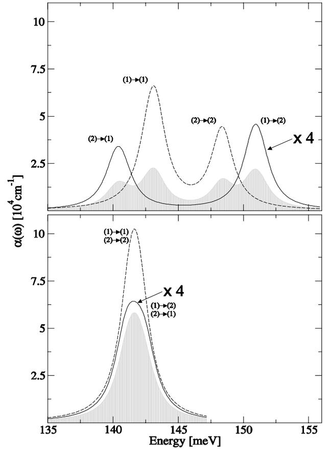
Fig.4: Intersubband absorption spectra for the Ge-QW system. Top (bottom) panel refer to well width of 37 (38) monolayers, corresponding to a maximum (minimum) in the valley splitting amplitude. Carrier concentration in the well region is  $8 \cdot 10^{12}$  cm $^{-2}$  per layer. Solid and dashed lines refer to normal and parallel incident light, respectively. Normal absorption is reported magnified by a factor 4. The grey shaded features represent the joint density of states.
