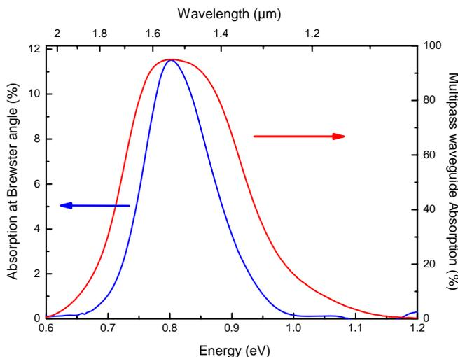
Figure 2: 300 K absorption spectrum at Brewster angle of incidence (blue curve) and in a multipass waveguide configuration (red curve).
