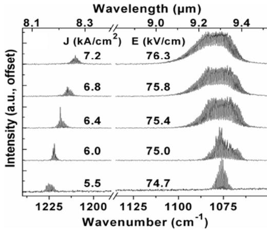
Fig. 3. Emission spectra of a 2.5 mm long and 10 μm wide laser at a heatsink temperature of 80 K operated with a 47 ns current pulse width. The electric field across the active laser core is calculated from current-voltage measurements.
