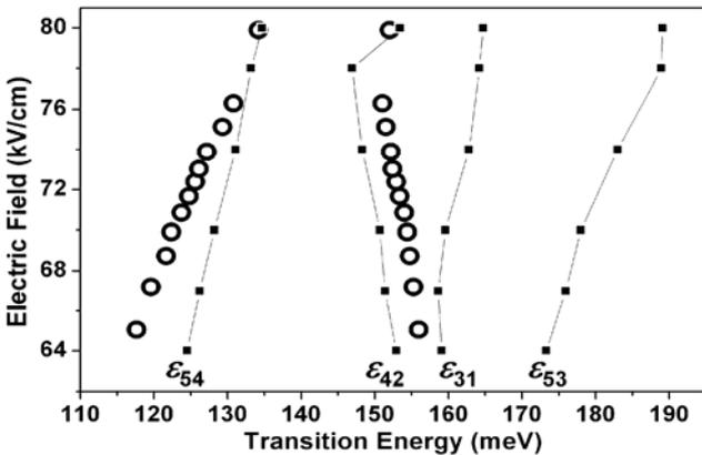
Fig. 4. Measured and calculated values of the optical transition energies in electroluminescence (EL) as a function of the electric field. Hollow circles represent the center points of multi-Lorentzian fits to the EL data. Solid squares show the calculated transition energies.
