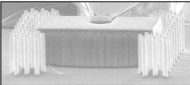
Fig. 1. Scanning electron microscopy picture of a microlaser with two-dimensional photonic crystals mirrors at both ends of the laser resonator.
