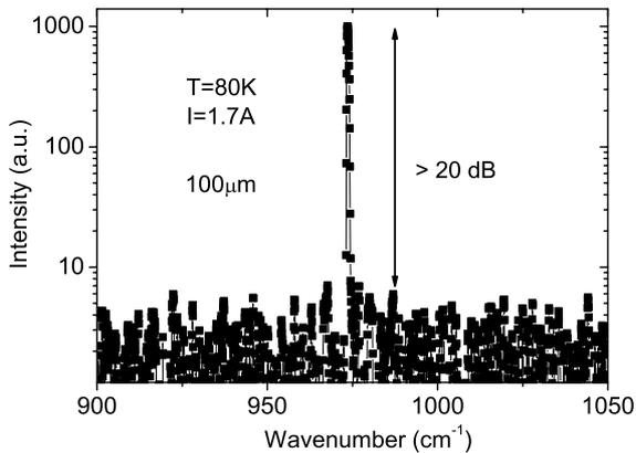
Fig. 3. High resolution singlemode spectrum of a 100  $\mu\text{m}$  long microlaser at 80 K.
