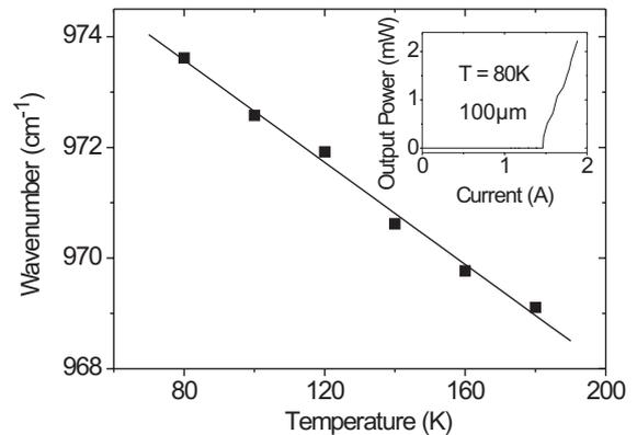
Fig. 4. Tuning behaviour of the emission wavelength of the 100  $\mu\text{m}$  long device with temperature. The inset shows a P-I-curve at 80 K.
