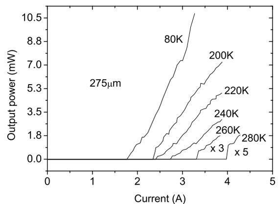
Fig. 2. Light output characteristics of a 275  $\mu\text{m}$  long microlaser. The P-I-curves at 260 and 280 K are re-scaled for better clarity.
