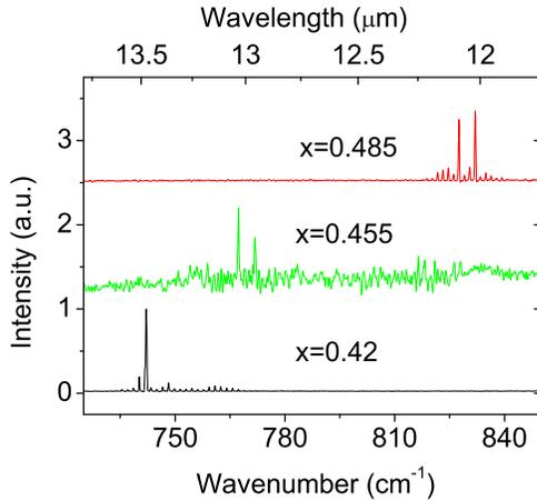
Fig. 2. Laser spectra for  $x=0.42$ ,  $x=0.455$  and  $x=0.485$  (from bottom to top).
