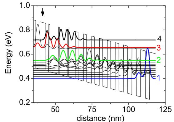
Fig. 1. Bandstructure for one period under an electric field of 33.5 kV/cm. The injection barrier is marked with an arrow. The layer sequence in nm (from left to right, beginning with the injection barrier) is **4.0/2.0/0.8/5.8/0.9/5.2/0.9/4.5/2.0/3.7/2.1/3.4/2.1/3.2/2.3/3.1/2.3/3.1/2.5/3.1/2.8/3.0/3.0/2.9/3.25/2.85** whereas barriers are printed in bold. Underlined layers are doped to a sheet carrier density of  $8.3 \cdot 10^{11} \text{ 1/cm}^2$ .
