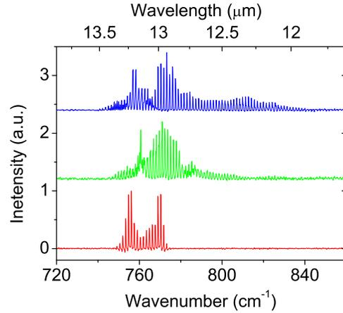
Fig. 3. Emission spectra for current densities of 17.6, 34.8 and 51  $\text{kA}/\text{cm}^2$  (from bottom to top) at a heat-sink temperature of 80K. For  $J=51 \text{ kA}/\text{cm}^2$  (top) broad-band emission from 740 to 840  $\text{cm}^{-1}$  is observed.
