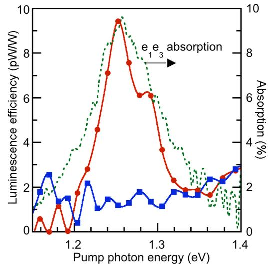
Fig. 3. ISB luminescence efficiency of sample B versus pump photon energy at room temperature for p- (circles) and s- (squares) polarized excitation (full curves). Right scale:  $e_1e_3$  absorption spectrum of sample B (dotted curve).
