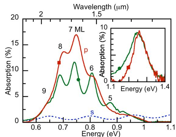
Fig. 1. Absorption spectrum at 300 K of samples B (squares) for p- and s-polarized light and A (circles) for p-polarized light at Brewster's angle of incidence. The inset shows the  $e_1e_3$  absorption for p-polarized light of samples B (squares) and A (circles) measured in a multi-pass waveguide.
