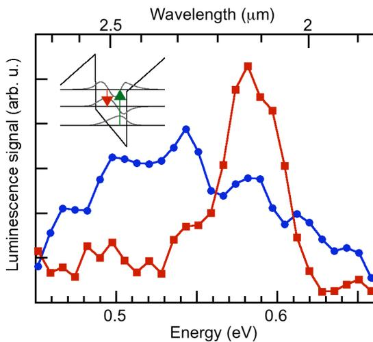
Fig. 2. ISB luminescence spectrum at 300 K of samples A (circles) and B (squares) under excitation at  $\lambda=0.98 \mu\text{m}$  wavelength. The spectra have been corrected for the spectral response of the optics, filter and detector. The inset shows the conduction band profile and energy levels of an 8 ML thick QW.
