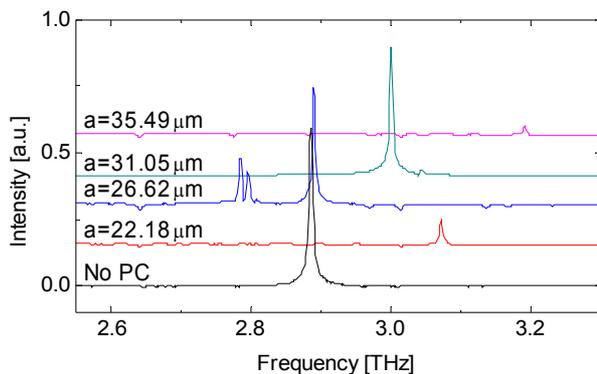
Fig. 3. Spectra of sample (a) with and without PC. The period of the PC has been varied from 22.18 to 35.49  $\mu\text{m}$ . The emission is shifted from the gain maximum of the active region into the bandgap.
