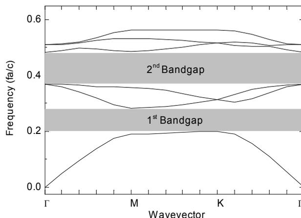
Fig. 1. Calculated bandstructure of the PC. The first two bandgaps for TM-modes are shown.
