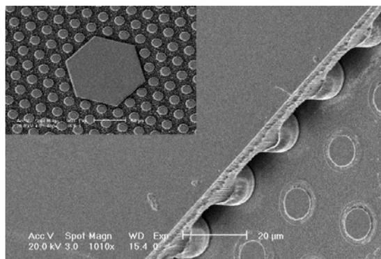
Fig. 2. Photonic crystal resonator after the wafer bonding. The thickness of the waveguide is 15  $\mu\text{m}$ . The inset shows the core and the surrounding PC before the wafer bonding.
