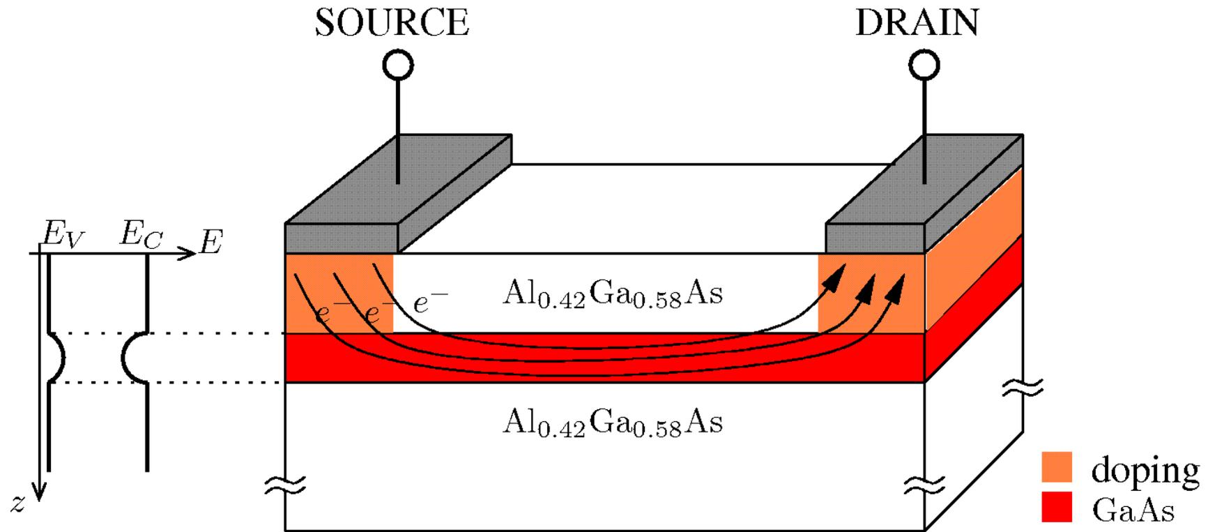
FIG. The possible construction of the laterally pumped quantum well emitter. The doping (e.g.  $10^{12} \text{ cm}^{-2}$ ) should be localised in 2D quantum layer and in the regions under the contacts. The quantum well layer, marked by red, actually contains a fine structure of potential barriers and wells created by  $\text{GaAs}/\text{Al}_{0.42}\text{Ga}_{0.58}\text{As}$  composition changes in  $z$ -direction. Approximate width of the QW layer is 60 nm.
