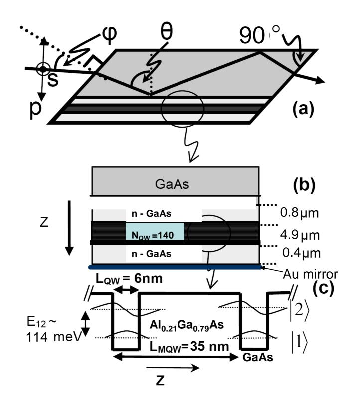
Figure 1: The prism coupling scheme (a) and the details of the metal clad microcavity structure studied in Ref. [1] (b,c).
