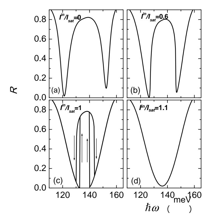
Figure 4: The spectral shape of R calculated for the structure presented in Fig. 2 at different values of  $I^{\rm in}/I_{\rm sat}$ .  $N_s \times f_{12} = 10^{11}~{\rm cm}^{-2}$ ,  $\hbar\Gamma = 3.8~{\rm meV}$ ,  $\theta = \theta_{\rm res} = 67.91^{\circ}$ .
