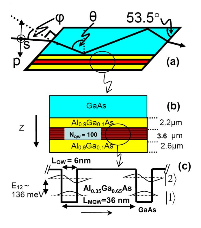
Figure 2: The prism coupling scheme (a) and the details of the dielectric microcavity similar to studied in Ref. [2] (b,c).
