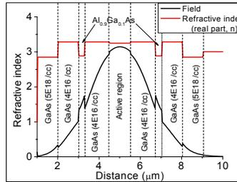
Use of  $\text{Al}_{0.9}\text{Ga}_{0.1}\text{As}$  cladding increases the optical confinement factor ( $\Gamma$ ) to compensate for the reduced number of stages
