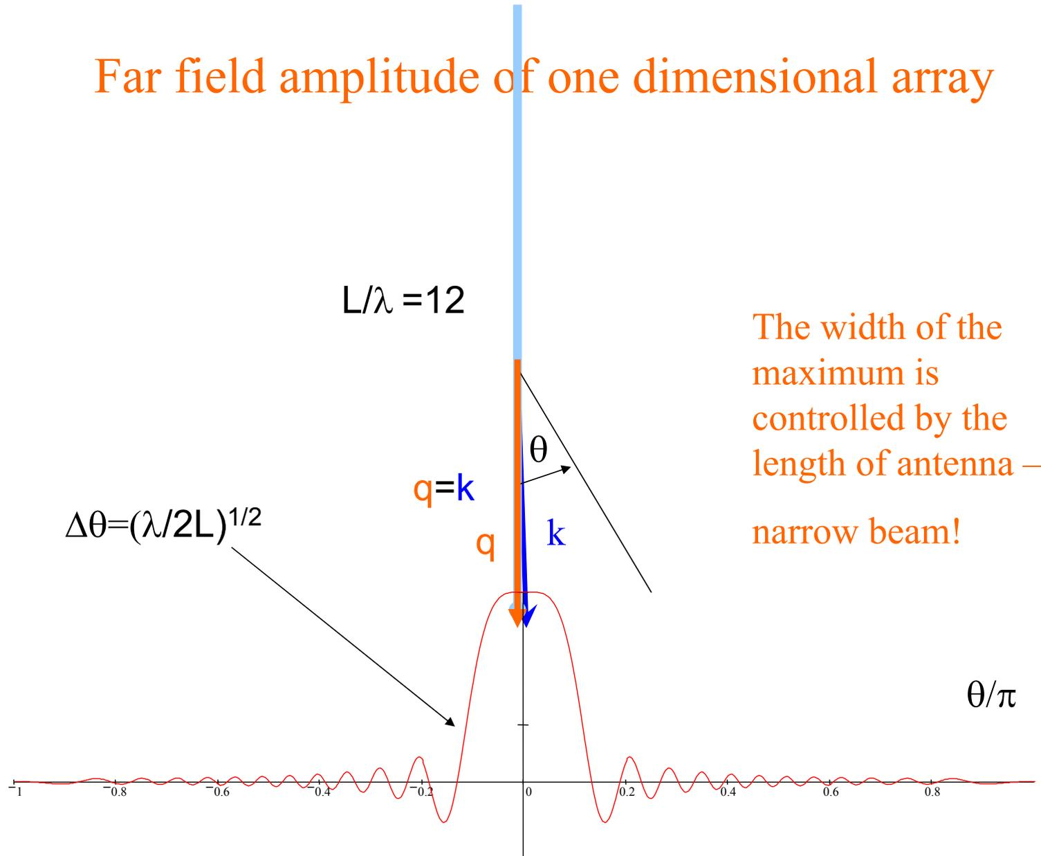
The width of the maximum is controlled by the length of antenna – narrow beam!
